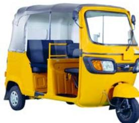
TVS King got a new variant in May 2019, with the introduction of TVS King Duramax with alternate fuel options like Petrol, LPG and CNG. This new variant comes with the 225 cc engine equipped with latest Liquid cooled technology, providing a great combination
